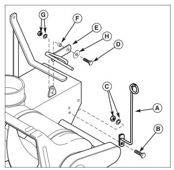
Figure 14. Deflector Control Cable Support Arm
